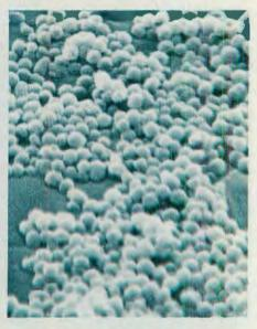
Tri-Flon Teflon® particles, without fluid boundary film, are enlarged 20,000 times to show "bearing-type" filling effect of submicron size particles. Millions of these particles are suspended in each milliliter of Tri-Flon.
